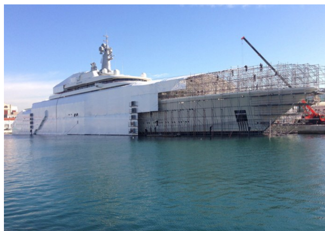
Scaffolding and tenting typically used by GYG in its repainting contracts.
